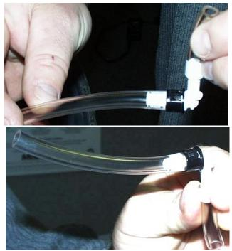
Take the FITTING-1/4 X 1/4 PLST 90 BARB (190421) and install a GROMMET (190403) onto one leg of the elbow. Take HOSE-1/4 ID X 8" LONG (190423) and install it onto the leg where the grommet was just placed. Then take HOSE 1/4 ID X 1.5 LONG (190420) and install it onto the open leg of the fitting.
