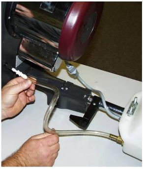
Press the ADAPTER 1/4 X 3/8 PLS (190422) into the HOSE-DUMP 24IN CLEAR C/L (430118). Then press the hose onto the FITTING-1/4FPT 3/8HOSE BRASS (833473) as shown at right.
