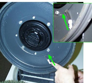
Install the tube assembly into the hole in the bottom of the housing (oriented toward the center hub) as shown above.
