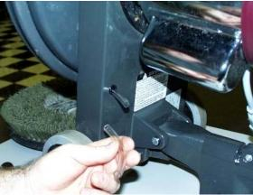
Slide the plastic sleeve onto the tube and into the hole (as shown above). Then trim the HOSE-1/4 ID X 8" LONG (190423) so that there is about 1-1/2" of tubing protruding from the frame.
